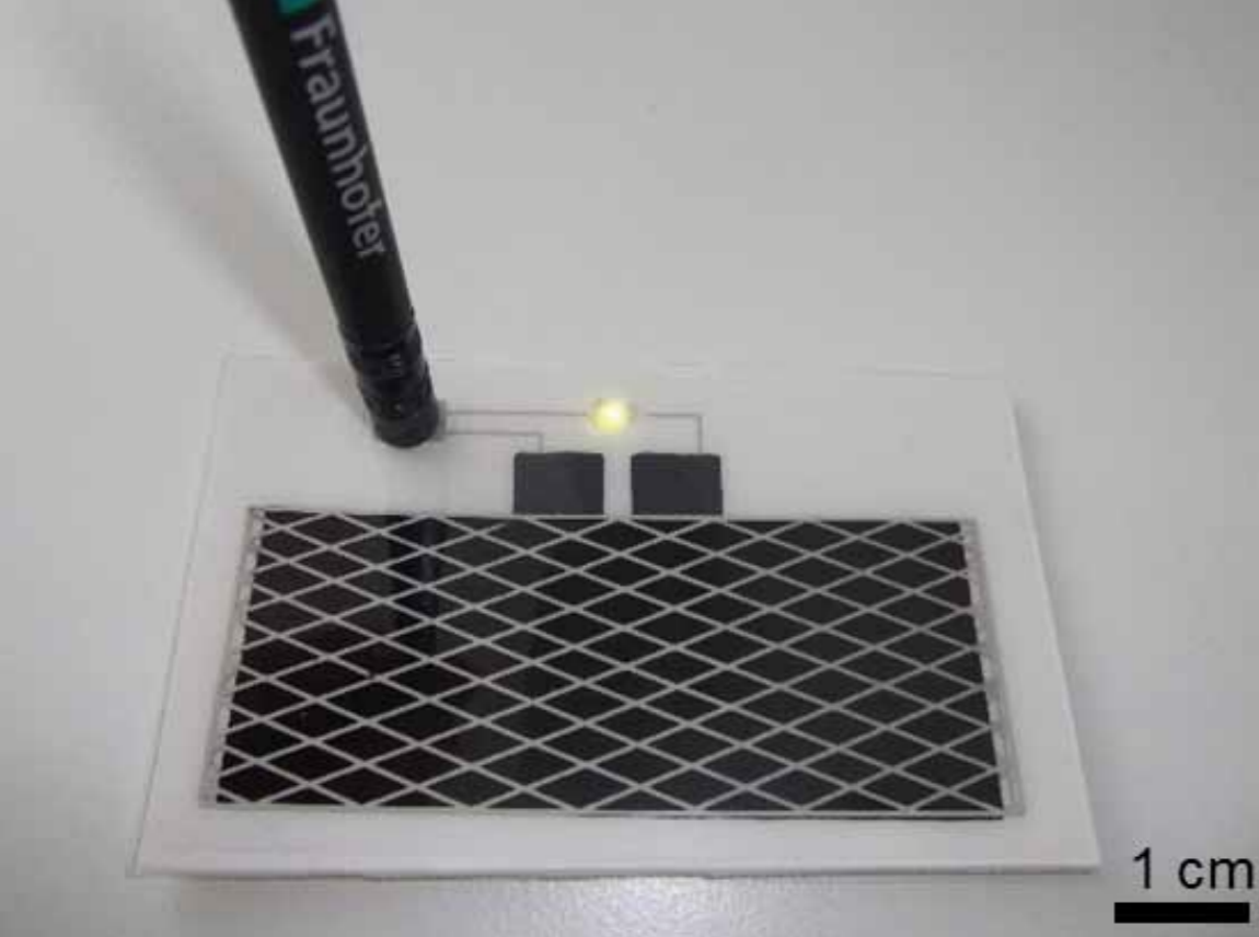
A printed battery manufactured on a technical textile driving one LED.
