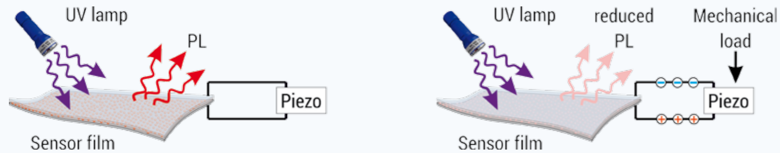
Sensor film with initial light intensity (left) and reduced intensity of sensor due to mechanical load (right).
