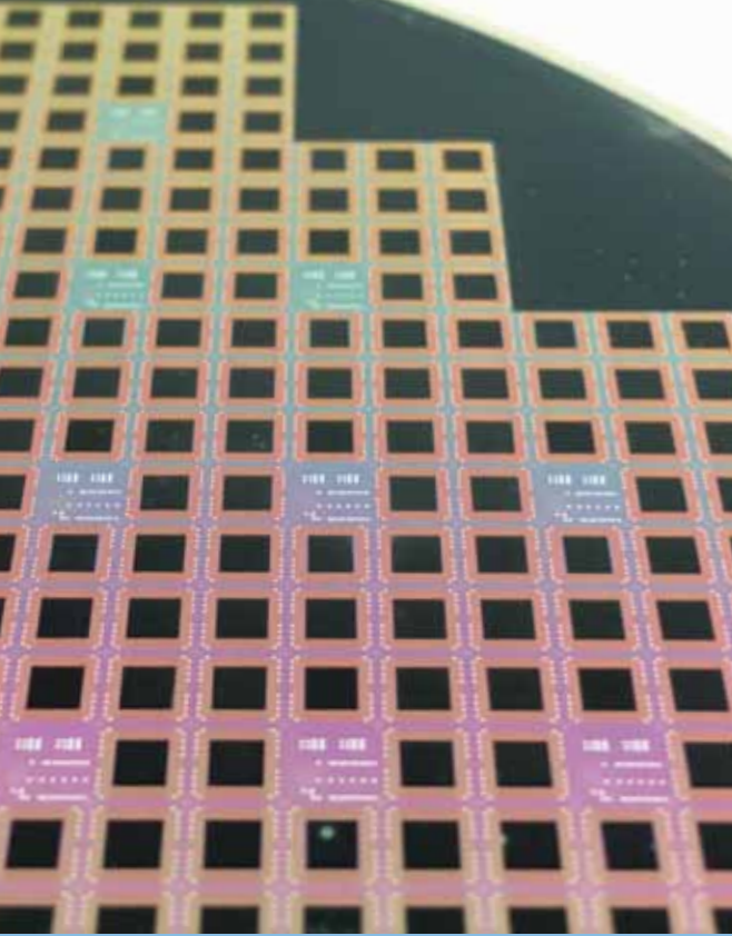
CNT absorption layers integrated in an IR emitter structure (left) and the absorption behavior of such CNT layers (right).
