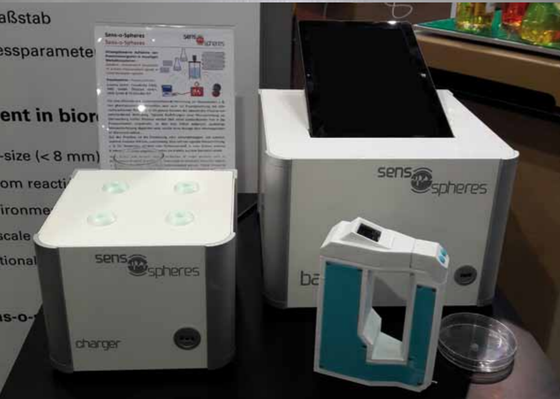
The Sens-o-Spheres demonstration system for wireless monitoring in different types of biotechnical mediums.
