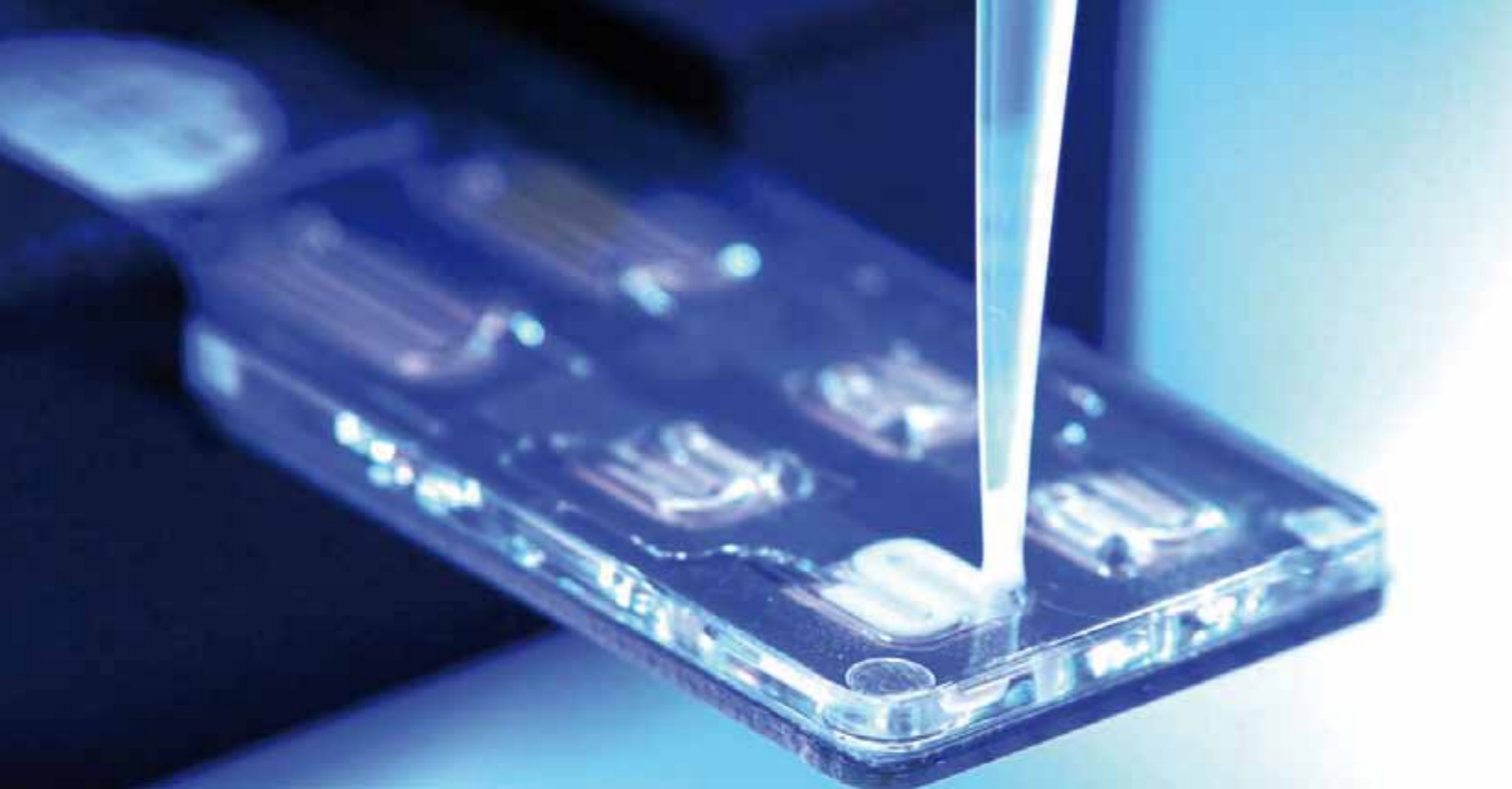
A milk sample is introduced into a microfluidic cartridge for analysis.
